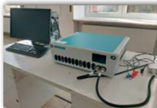
Sistem electrochimic multi-modular Autolab 128N
