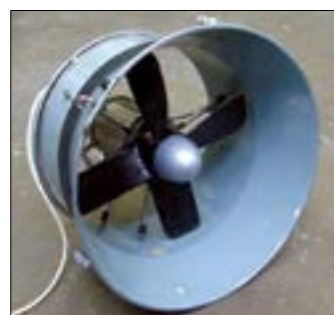
Microhidrogenerator electric intubat
